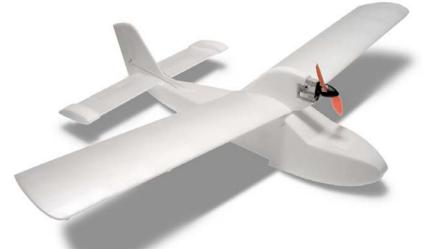
Electric Foam Parkflyer with "Slot and Groove" construction.
