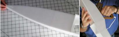
f) To fit the top in place, cut or sand a bevel towards the front of the top where it meets the form so that it will fit flush. The groove on the fuselage top and front faces the inside of the fuselage. Bend the top away from the groove to form the angle where the "rear window" meets the fuselage top. When the fit is good, glue the top rear section in place.
