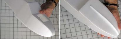
h) If you wish, the keel can be glued to the bottom of the forward fuselage centered on the underside of the hull. This would help with handling on snow and water. If you'll be flying almost entirely off of land, then it isn't really necessary except for looks...
