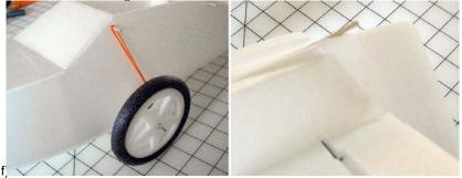
The landing gear can be added and removed any time you like simply by removing the rubberbands.
